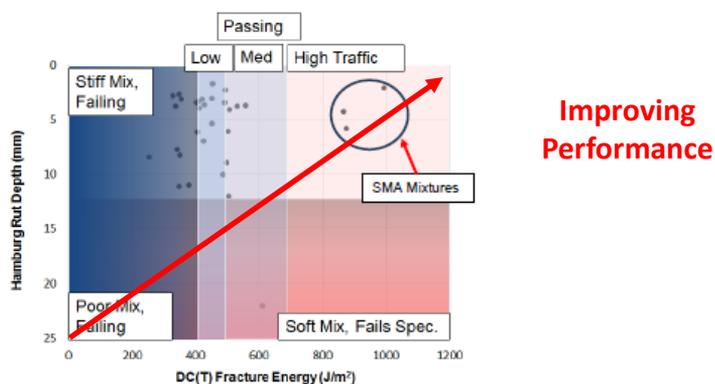
Figure 12. Hamburg-DC(T) Plot for Recent Mixtures Tested in Illinois, with Typical Specification Limits Superimposed.
